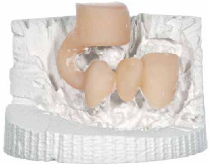
Bridge with one 4-mm sprue.
